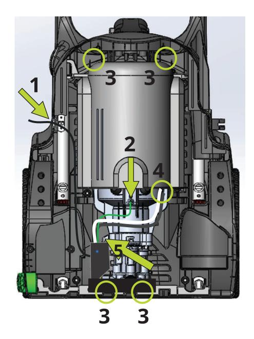
You must loosen the motor and pump to be able to unscrew the electrical box:
